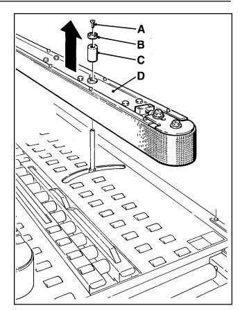
Figure 6-1 – Drive Belt Height, Disassembly
